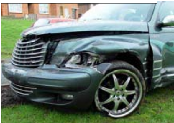
Front-end 70mph damage, steering broken, radiator back about 2 feet
